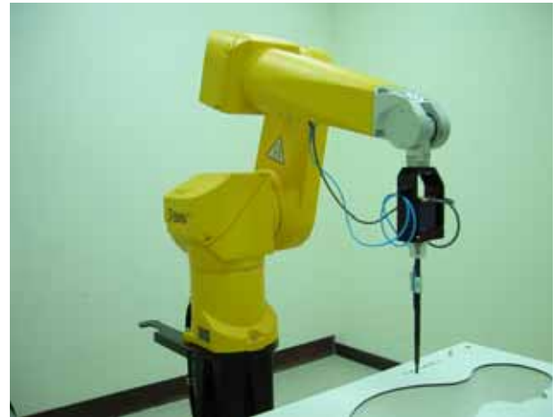
Fig. 5.3 Probe setup on robot
