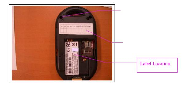
The label will be placed under the battery compartment, and it's visible to the users as they purchase the product and install the battery.
