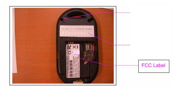
The label is placed inside the battery compartment.
