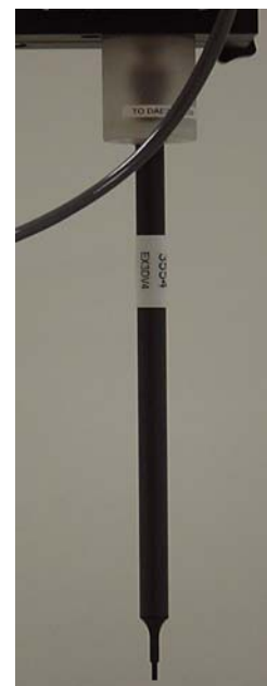
E-Field probe EX3DV4
