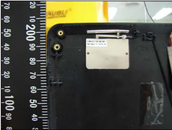
Aux antenna to user distance (116mm=11.6cm)
