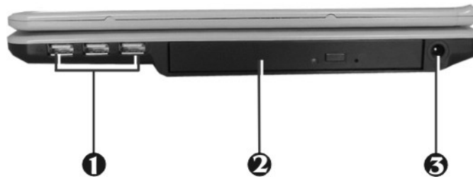
1. USB 2.0 Ports 2. Optical Disk Drive 3. DC Power Port
