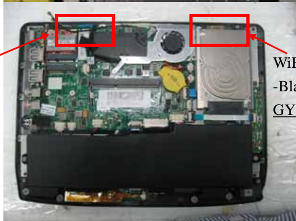
Bluetooth Antenna -White cable GY196C098-031
