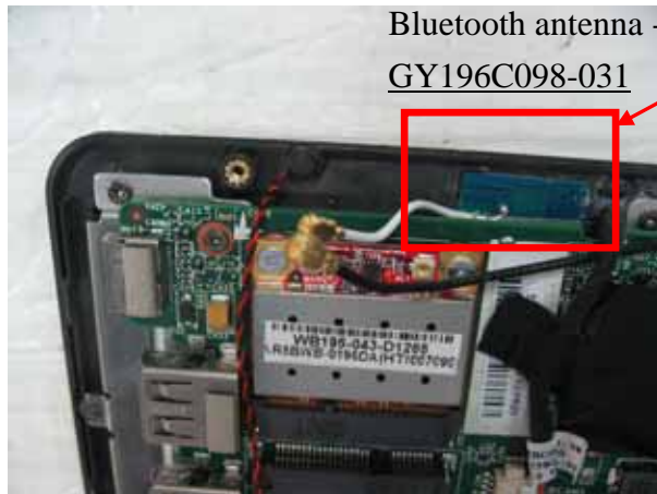
WiFi 2.4GHz Antenna - black cable GY196C098-032
