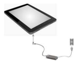
Whenever possible, it is advisable to always have the AC adapter connected to the Tablet PC. This ensures continuous power supply and prevents any data loss incurring from sudden power breakdown.
