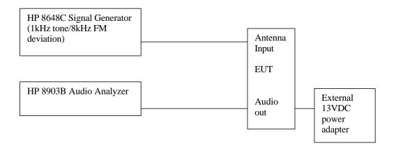
Frequencies used on the Signal Generator were 824.04, 836.50, 848.97 MHz for the Mobile and 881.50, 869.04, 893.97 MHz for the Base.
