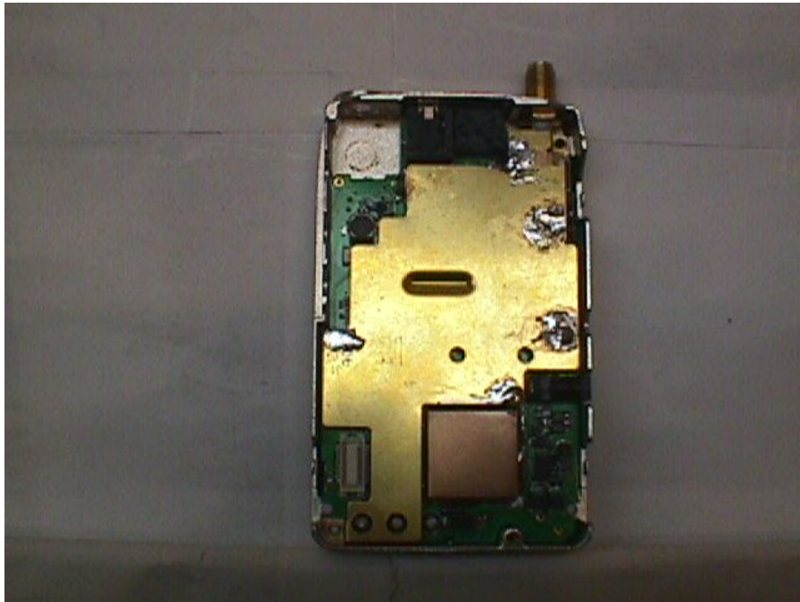
FIGURE 16: Main Board with copper shield
