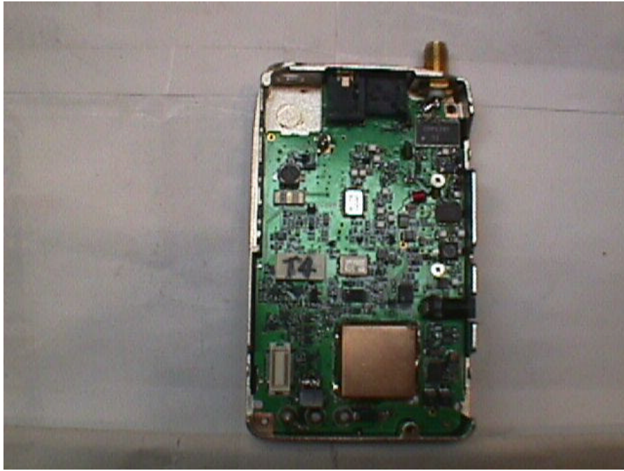
FIGURE 17: Main Board without copper shield
