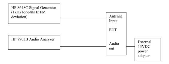
Frequencies used on the Signal Generator were 824.04, 836.505, 848.97 MHz for the Mobile and 869.04, 881.505, 893.97 MHz for the Base.
