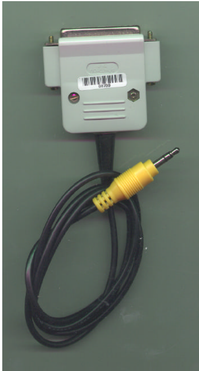
FIGURE 12: Service Port Cable
