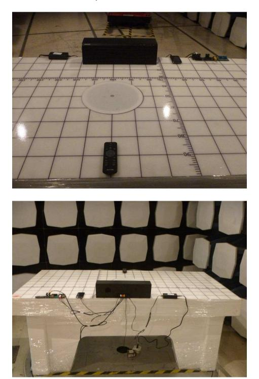
Test Setup Photo –Radiated Emission
