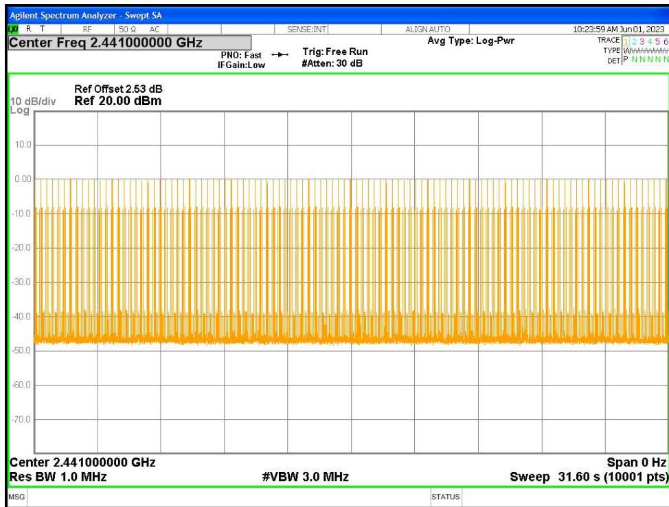
Dwell NVNT 2-DH1 2441MHz Ant1 One Burst
