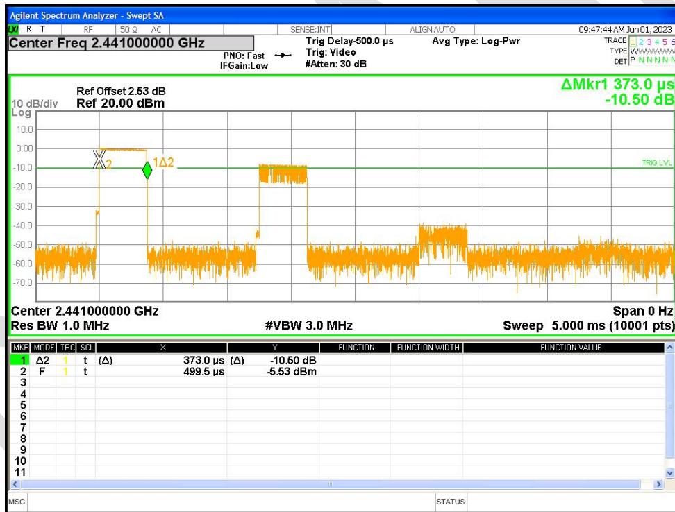
Dwell NVNT 1-DH1 2441MHz Ant1 Accumulated
