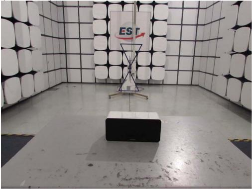
Radiated Test (1000-25000 MHz)
