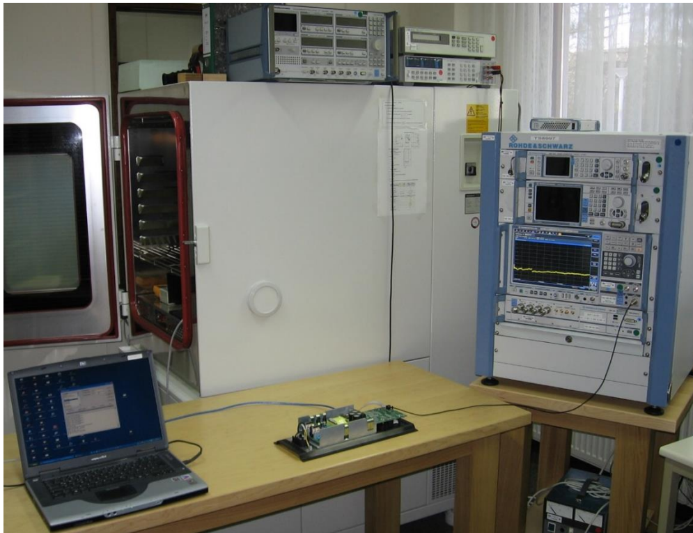
spurious emission conducted with spectrum analyzer
