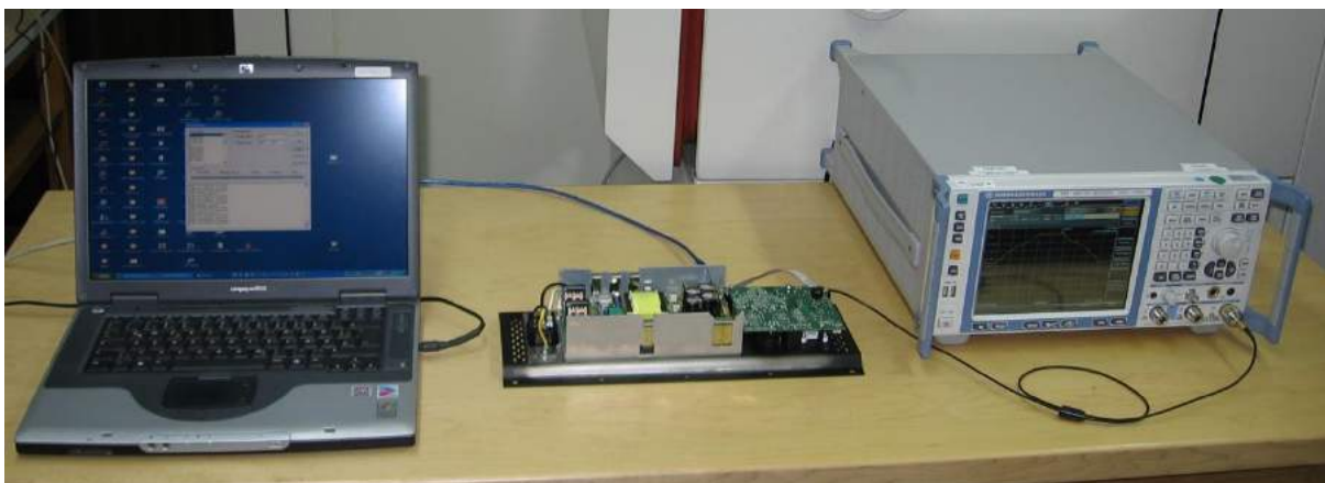
20 dB bandwidth, 99 % bandwidth, hopping channel separation, hopping channel frequencies, time of occupancy, Maximum peak conducted output power, Conducted RF band edge emissions with ESR7 EMI Testreceiver
