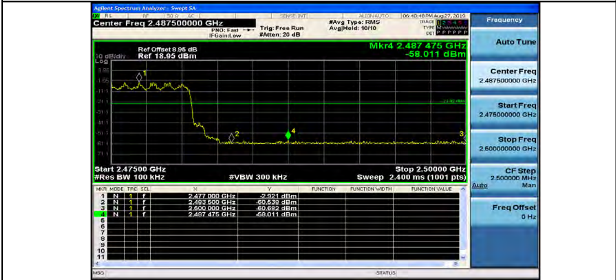
Band-edge for RF Conducted Emissions_2DH5_2480_Hopping Off
