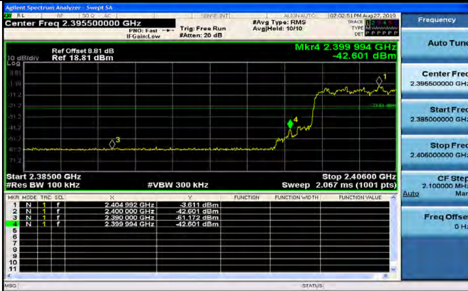
Band-edge for RF Conducted Emissions_3DH5_2402_Hopping Off
