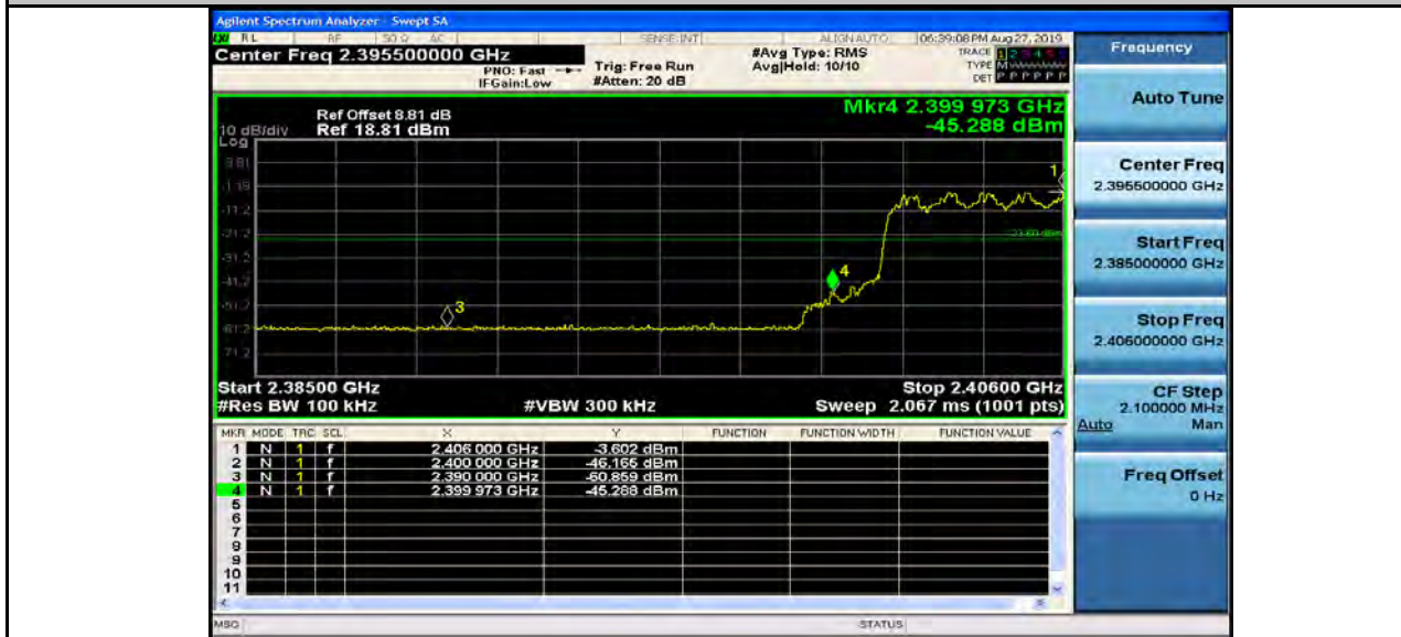
Band-edge for RF Conducted Emissions_2DH5_2402_Hopping Off
