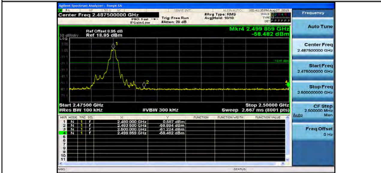
Band-edge for RF Conducted Emissions_2DH5_2402_Hopping On
