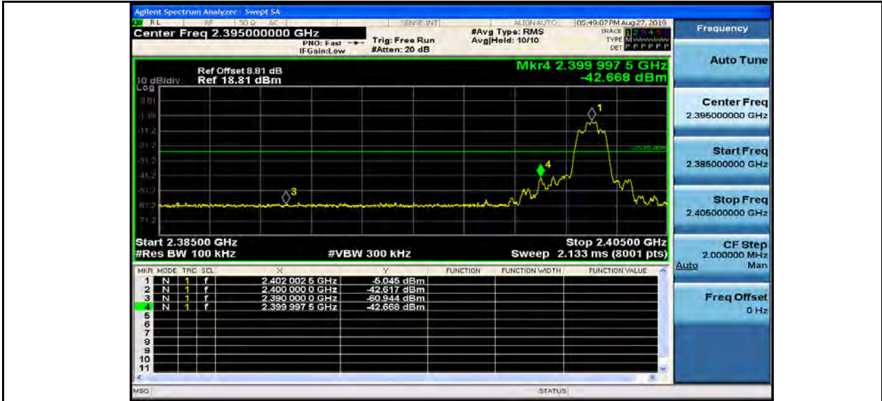
Band-edge for RF Conducted Emissions_2DH5_2480_Hopping On
