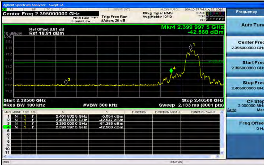
Band-edge for RF Conducted Emissions_3DH5_2480_Hopping On
