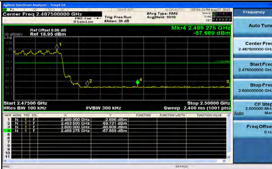
Band-edge for RF Conducted Emissions_3DH5_2480_Hopping Off
