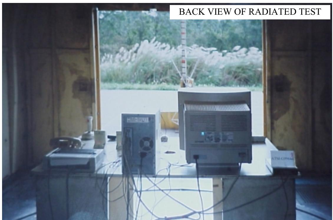
SETUP WITH MAXIMUM DETECTED EMISSION
