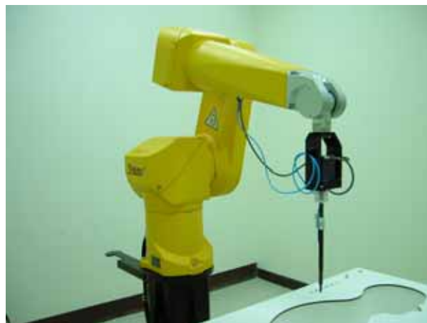
Fig. 5.2 Probe setup on robot
