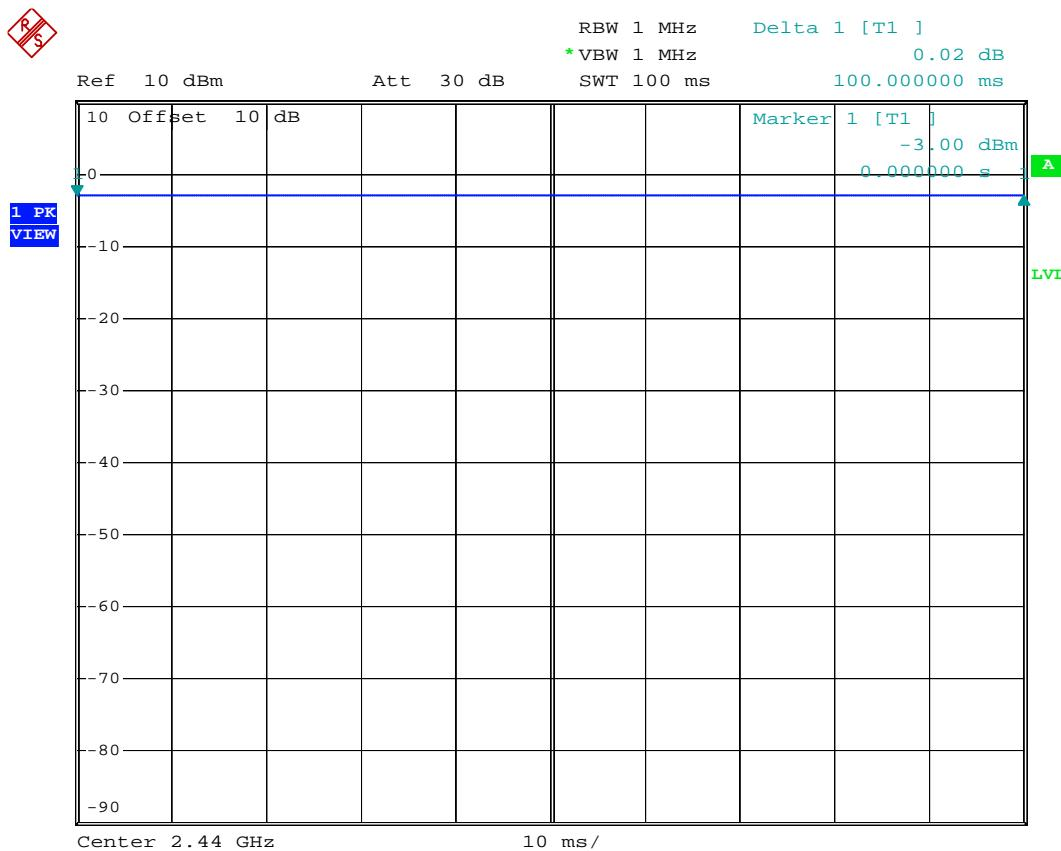
The EUT set for test with the continuous transmission mode and the duty cycle >98%.
