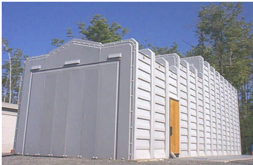
Fig. 1.b APREL's OATS (Open Area Test Site)
