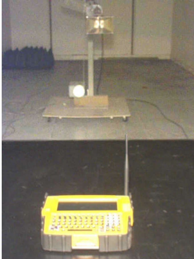
Melard Technologies Inc.'s Sidearm ALL-Terrain Handheld PC™ Tested for Spurious Emissions at the OATS
