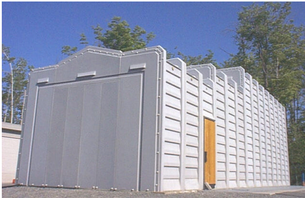
Fig. 1.b APREL's OATS (Open Area Test Site)
