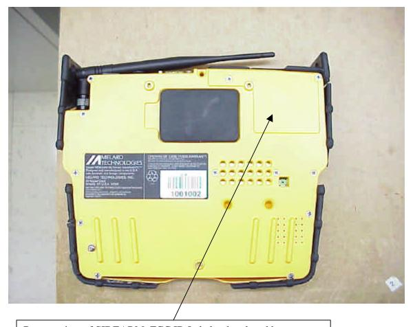
Bottom view of SIDEARM. FCC ID Label to be placed here.
