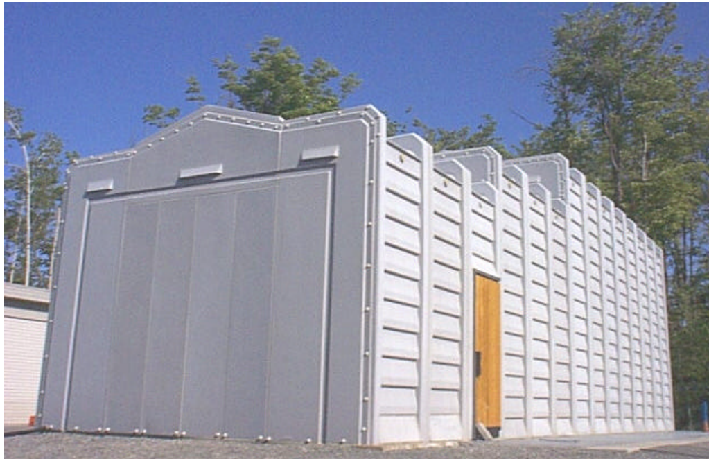
Fig. 1.b APREL's OATS (Open Area Test Site)
