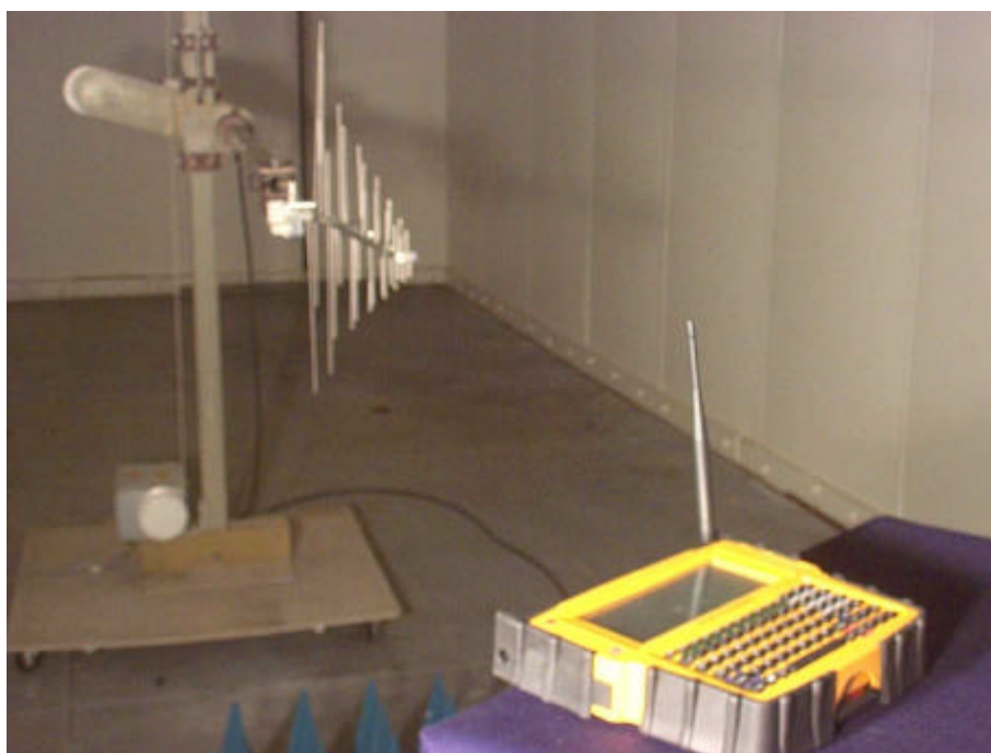
Sidearm ALL-Terrain Handheld PC™ Tested for ERP at the OATS
