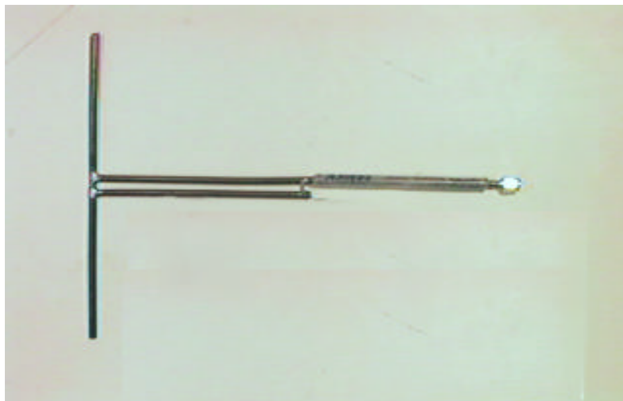
Reference Dipole Antenna Used for ERP Measurement
