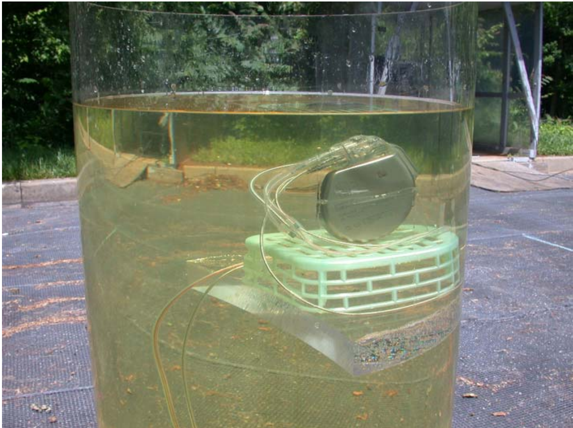
In- and out-of-liquid Radiated Test Photos
