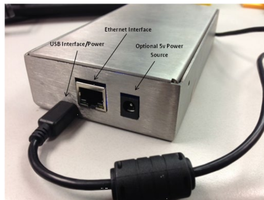
Figure 4: Fully Assembled System with Direct Connection for Ethernet
