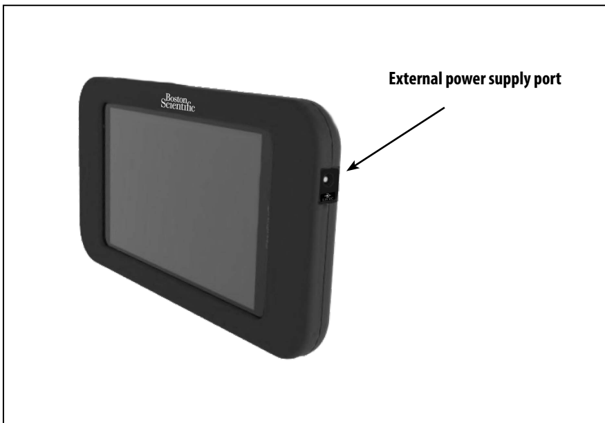
Figure 2: Connecting the external power supply
