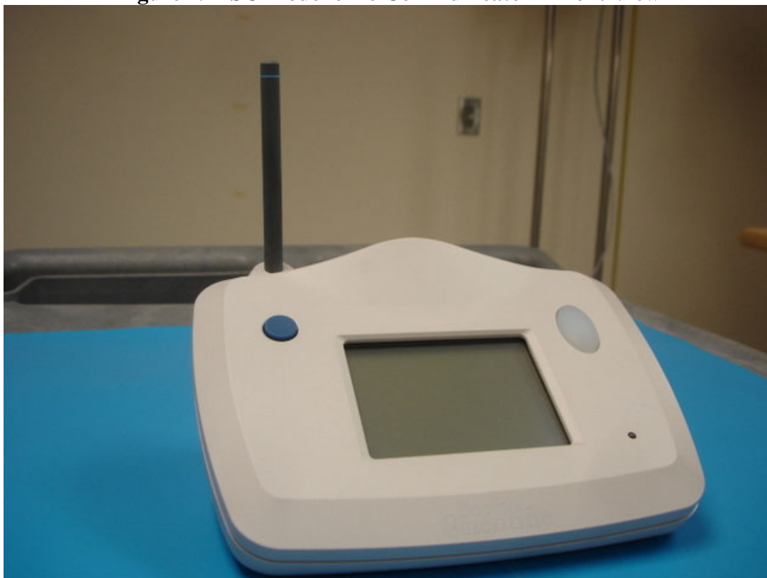
Figure 1. BSC Model 6476 Communicator - Front View
