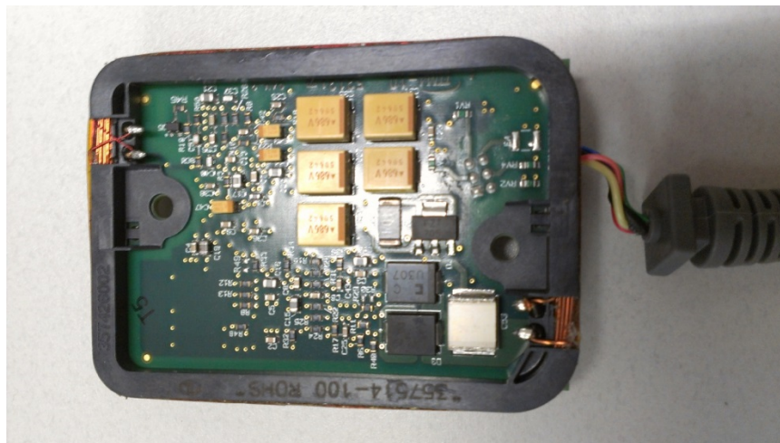
Figure 5. Wand Printed Circuit Assembly – Bottom Side (for reference only)
