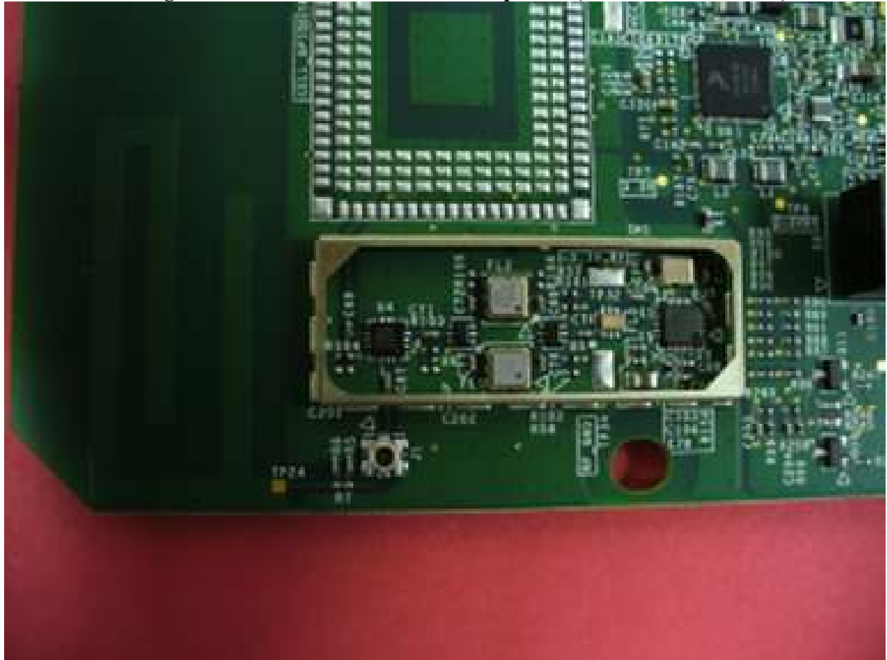
Figure 2 RF Transceiver Section – Top View (shield cover removed)
