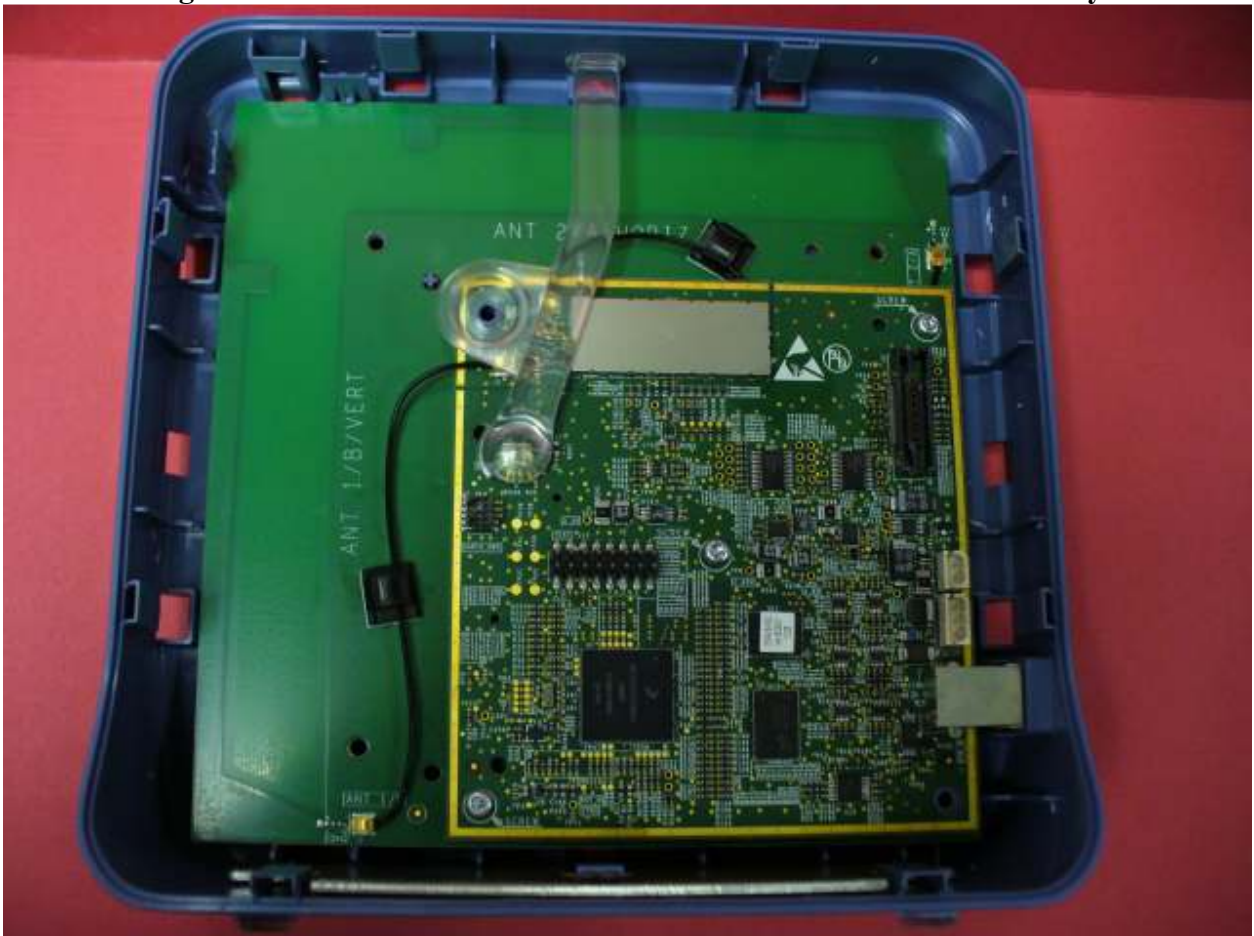
Figure 1 Model 3140 Zoom Wireless Transmitter – Internal Assembly
