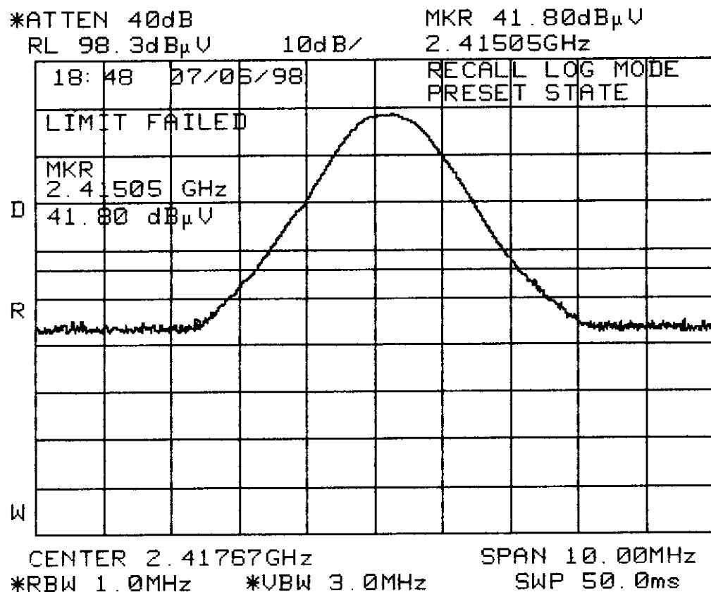
***Test Result of Harmonic Above 1 GHz :******(Horizontal)***
