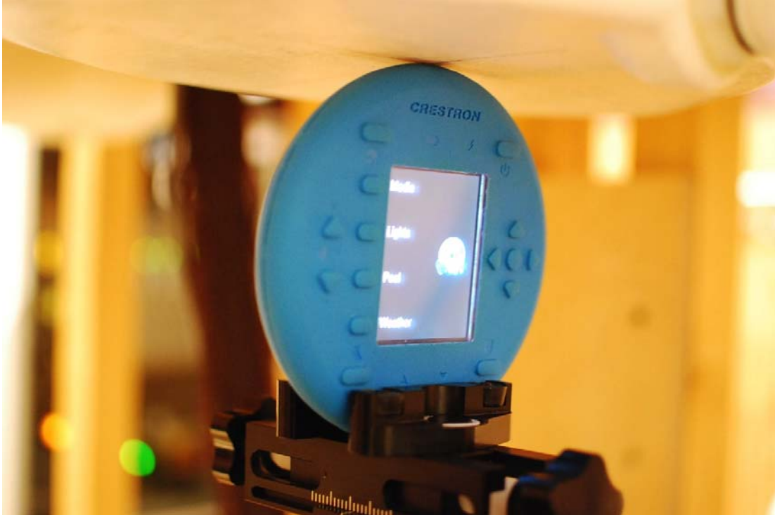
Figure 18-1 SAR Test Setup Photo 1: Top Edge
