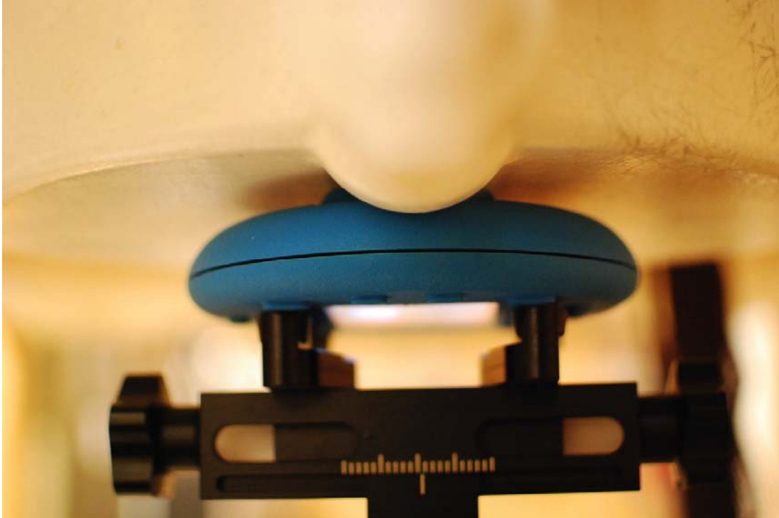
Figure 18-3 SAR Test Setup Photo 3: Back Side
