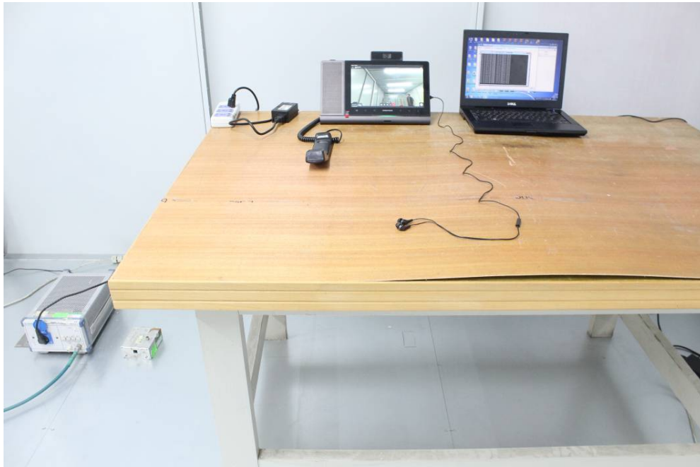
Conducted Emissions - Front View
