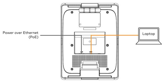
If using the included power supply to provide PoE to the UC-2, connect the supply as shown below.
