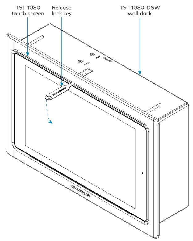
3. Remove the key to open the cradle so that the touch screen can be removed.
