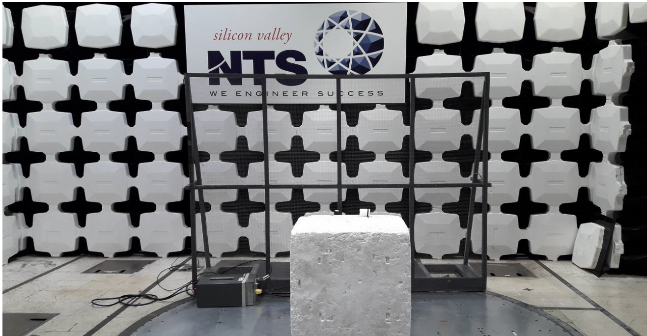
Test Configuration Photograph #1 (Conducted Emissions - Power Port)
