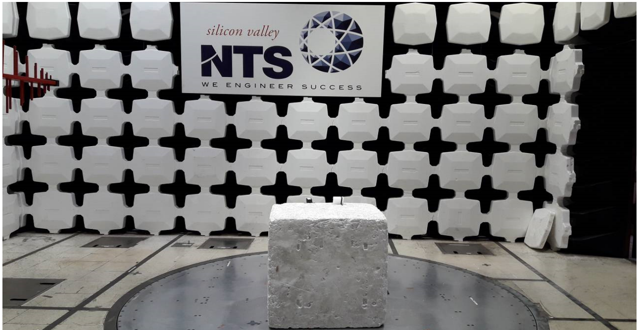
Test Configuration Photograph #3 (Radiated Emissions - Above 30 MHz)
