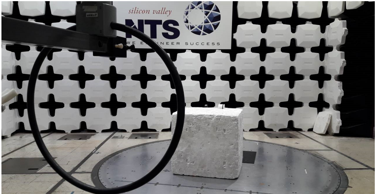
Test Configuration Photograph #1 (Radiated Emissions - Below 30 MHz)
