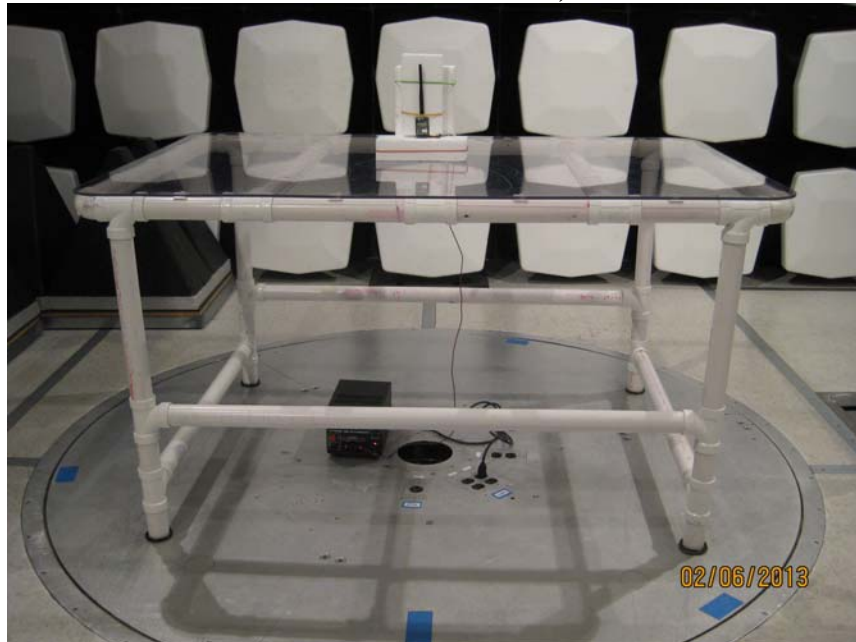
Worst-case radiated emission, front view
