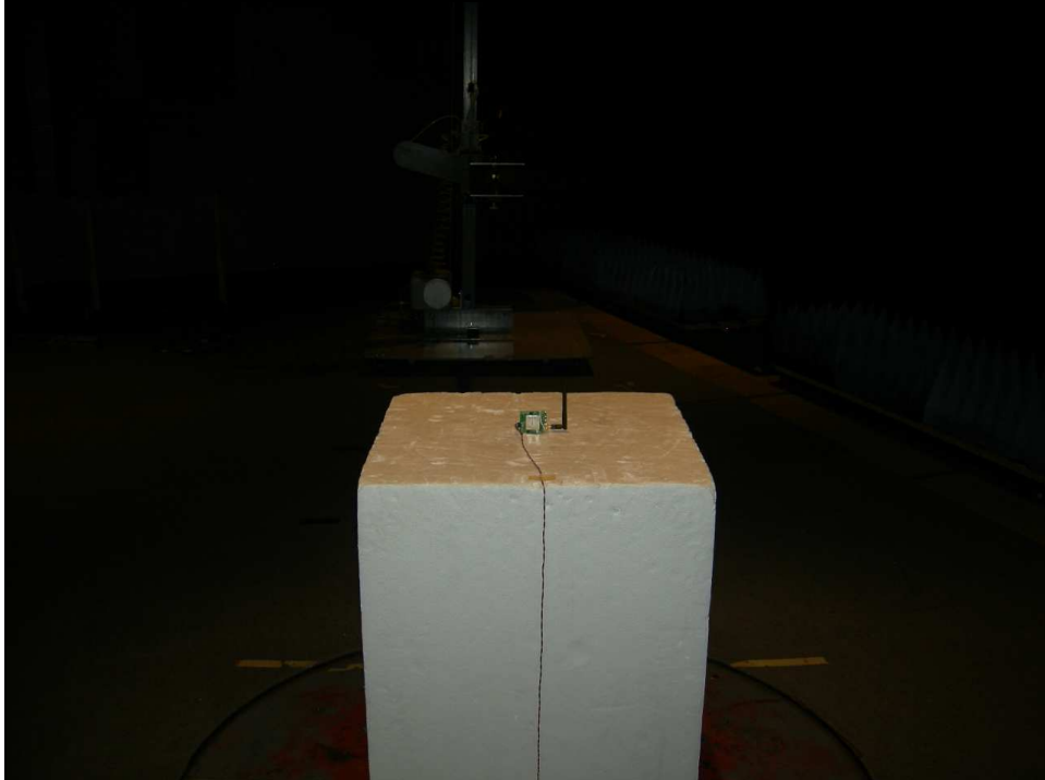
Figure 8: Radiated Emissions – Dipole Antenna – ZPOS
