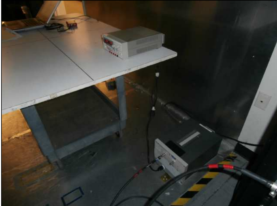
Figure 10: Conducted Emissions – Side View – Integrated Antenna
