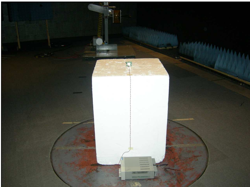
Figure 4: Radiated Emissions – Integrated Antenna – ZPOS
