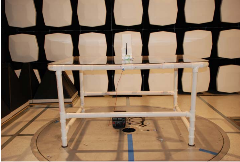
Worst-case radiated emission, front view
