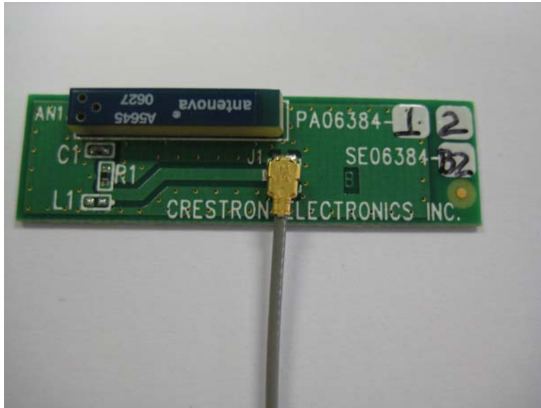
View of Antenna Connection (Crestron Cabled PCB Ceramic Chip Antenna U.FL Connector Type)
