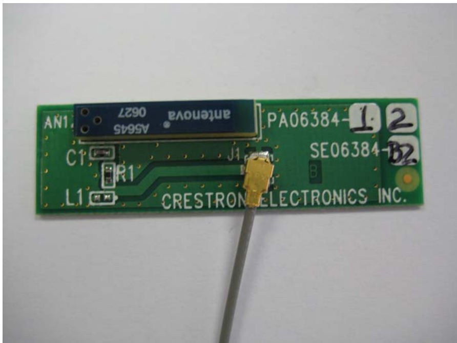
Back Side View #2 of Cabled PCB Ceramic Chip Antenna
