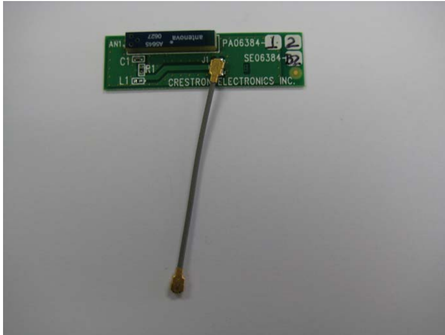
Back Side View #1 of Cabled PCB Ceramic Chip Antenna
