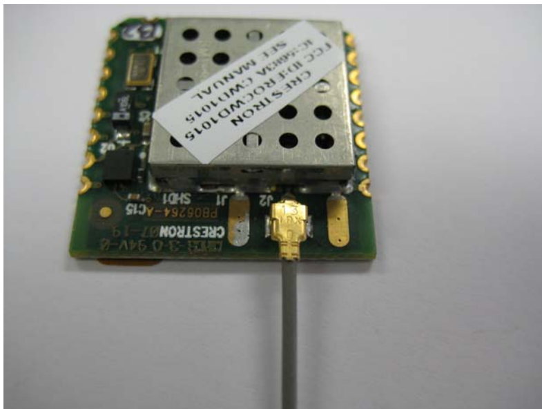
View of Antenna Connected to Module (Crestron Cabled PCB Ceramic Chip Antenna U.FL Connector Type)
