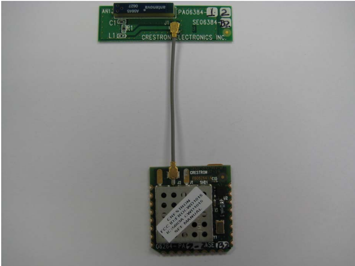
View # 2 of Module, with Crestron Cabled PCB Ceramic Chip Antenna Connected U.FL Connector Type. Cable measures 5 cm.
