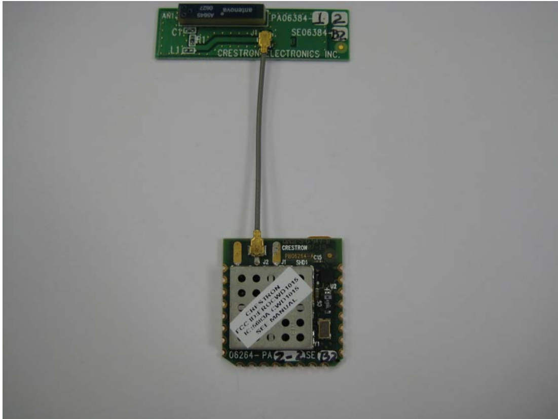
View # 1 of Module, with Crestron Cabled PCB Ceramic Chip Antenna Connected U.FL Connector Type. Cable measures 5 cm.
