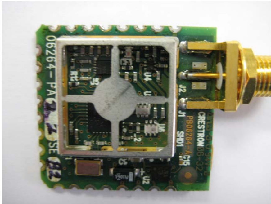
View #4 of RF Section, Shield Removed
