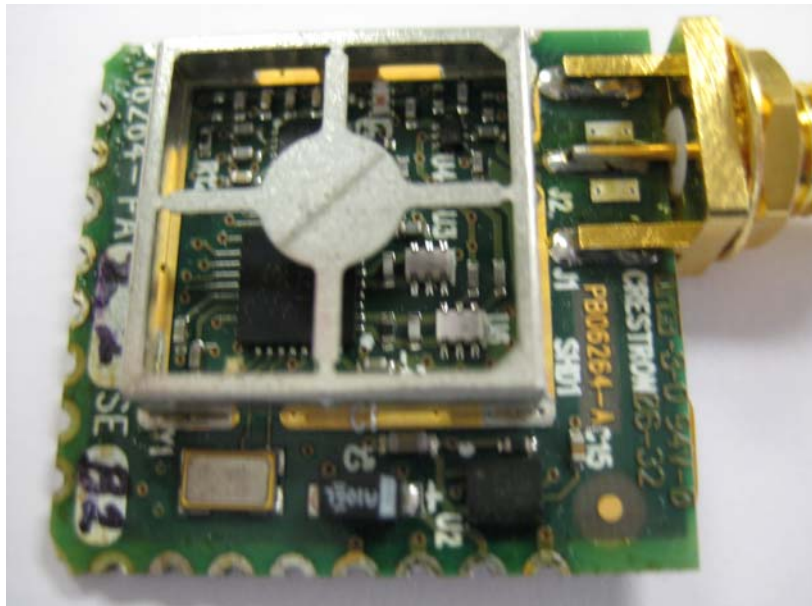
View #2 of RF Section, Shield Removed
