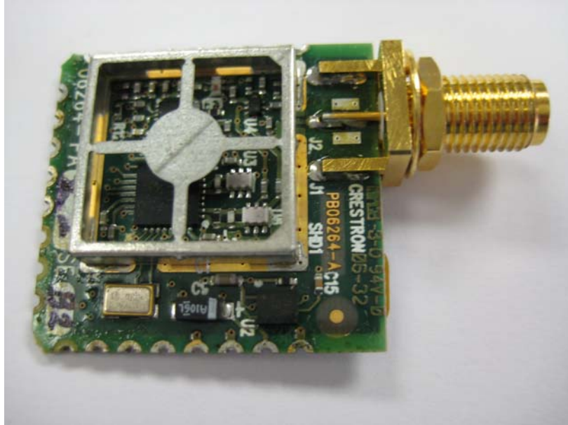
View #1 of RF Section, Shield Removed
