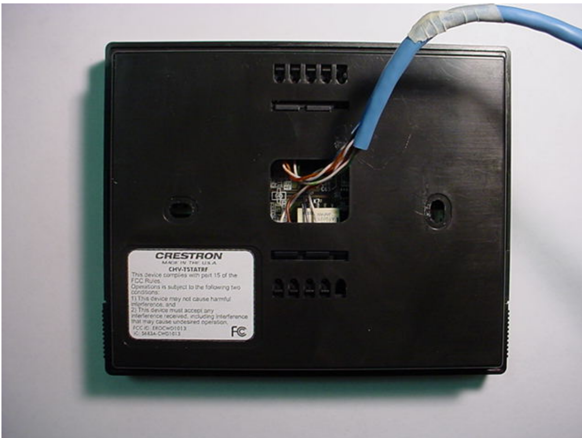
Photo Three – External Rear Panel with I/O Cable & Showing FCC ID Label
