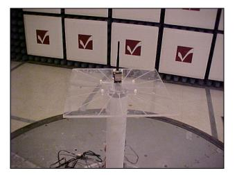
Setup for the Radiated Emissions Test
