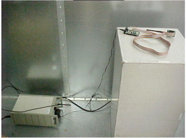
Setup for the Conducted Emissions Test
