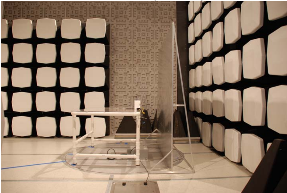
Worst-case conducted emission, Side View, LAN PoE Port
