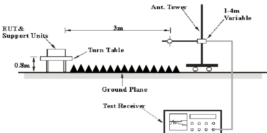
The radiated emission tests were performed in the 3 meters chamber test site, using the setup accordance with the ANSI C63.4-2014. The specification used was the FCC Part 15.109 limits.
