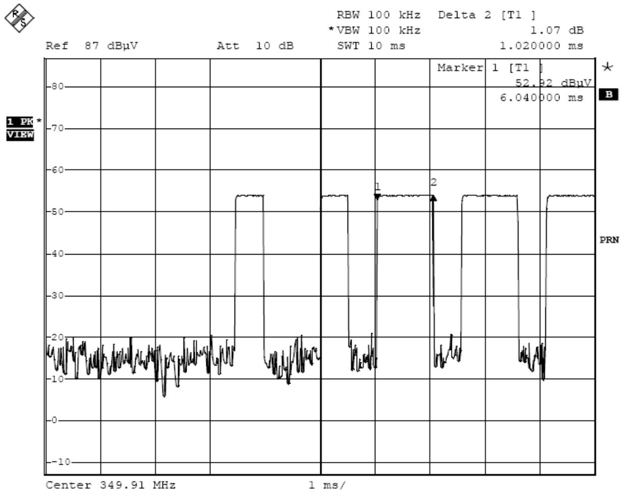
The graph shows the duration of long 'on' signal. From marker 1 to marker 2, duration is 1.02ms.
