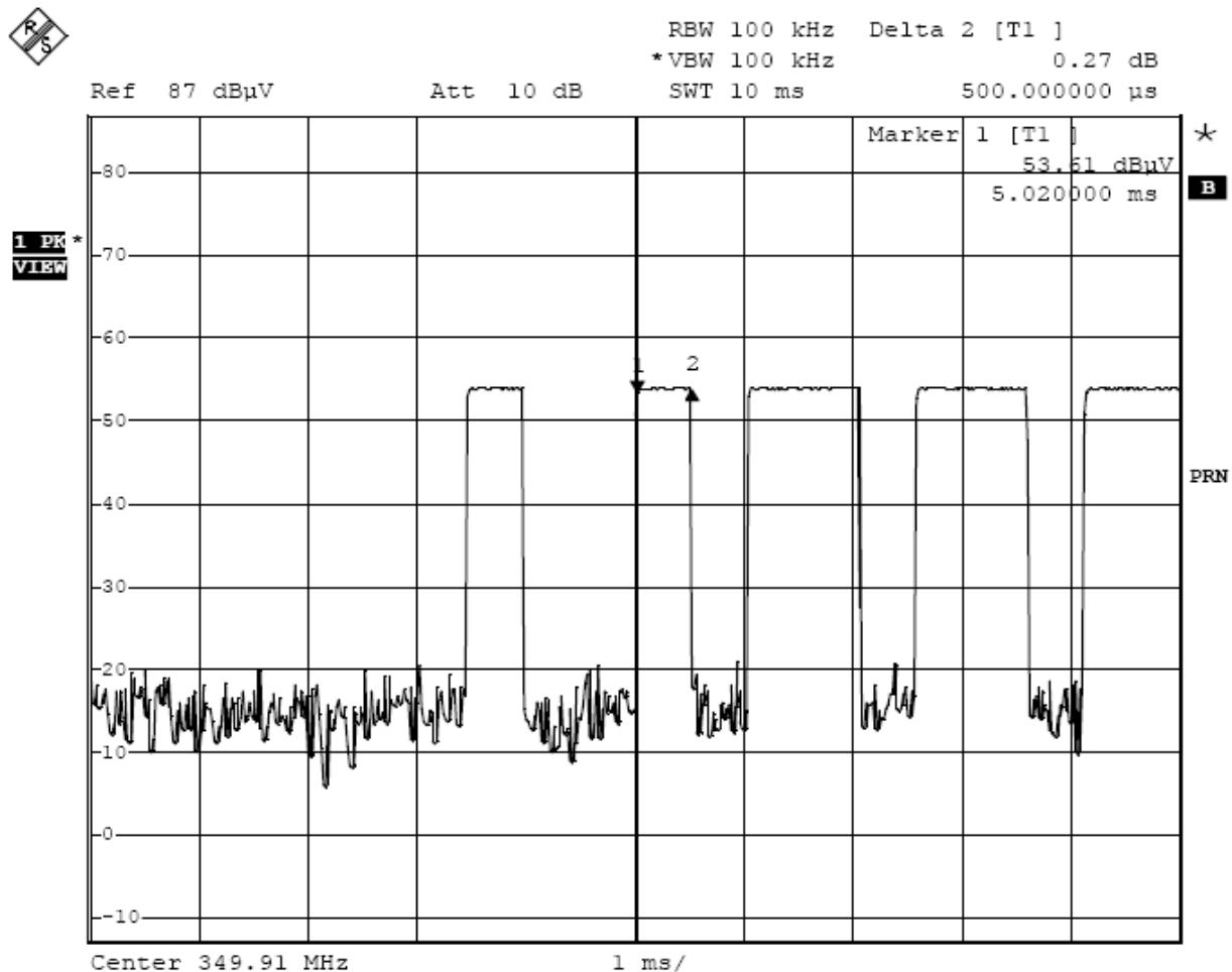
The graph shows the duration of short 'on' signal. From marker 1 to marker 2, duration is 0.5ms.
