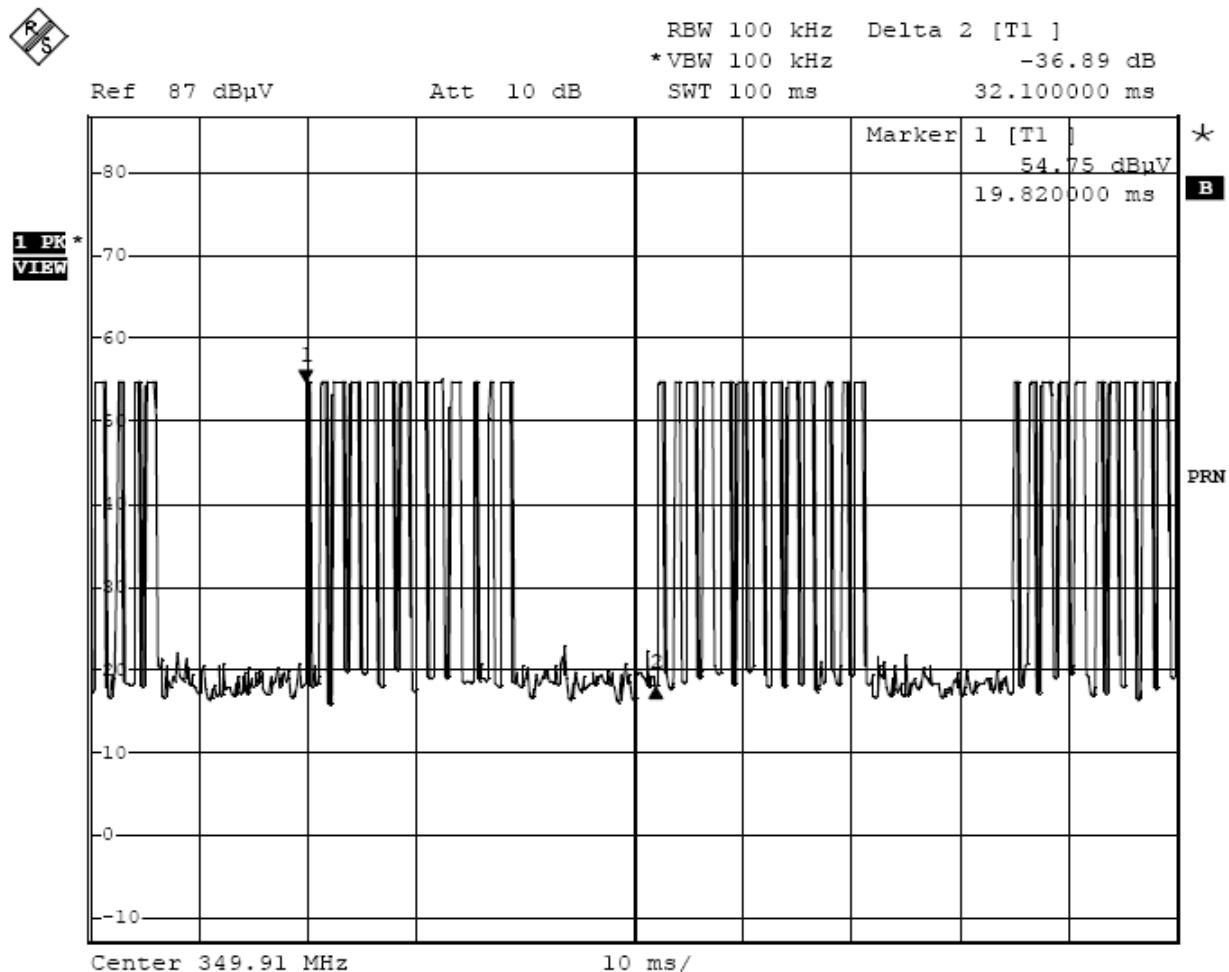
The graph shows the pattern of coding during the signal transmission. The time interval of one coding period starts from marker 1 to marker 2, Hence the total time of one period is 32.1ms. It sums of 9 long 'on' signals and 4 short 'on' signals.
