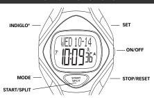
When setting, each button has a different function as indicated above. Display indicates when button changes function.
