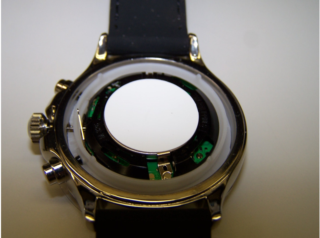
Figure 1: M329 with Case-Back in Removed.
