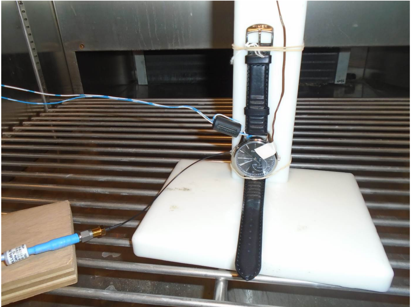
Figure 8 – View of EUT inside of Temperature test chamber for direct measurements. The Modular device on the watch host was modified with a coax and connector to allow direct measurements.
