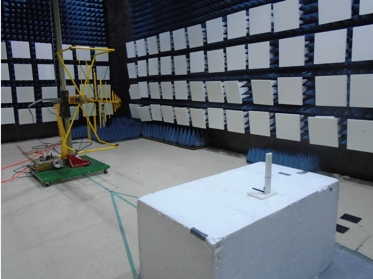
Figure 2: Typical Radiated Emissions – 30 MHz to 1 GHz shown, rear view. The Limited Modular Device is running in a typical application in a watch.
